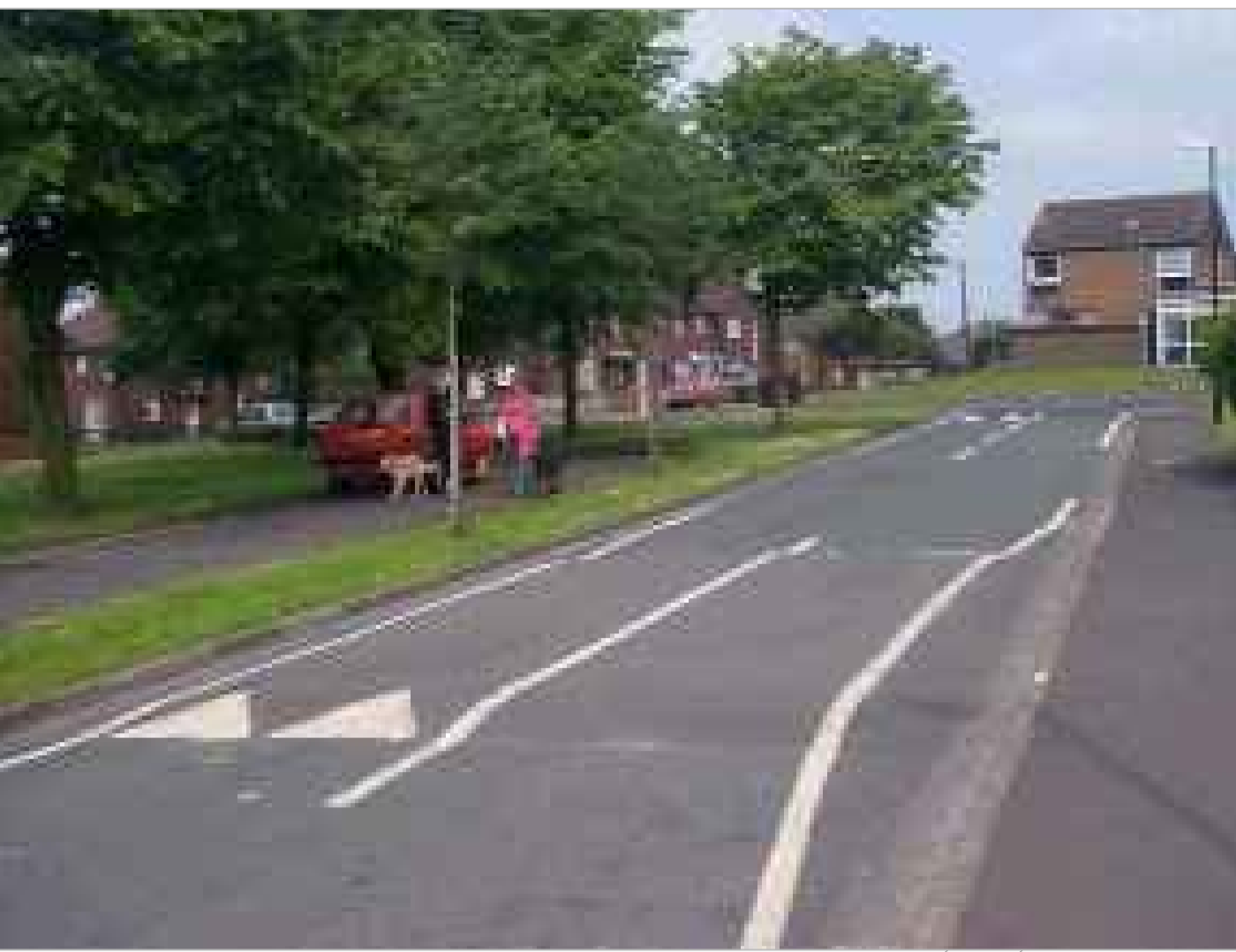
Example of Flat Topped Hump - West Bergholt Hump would not have the edge lining
